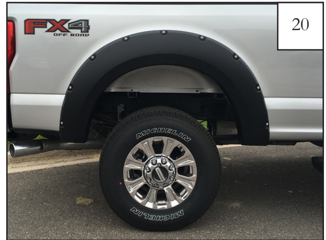
20 Completed rear flare installation.
