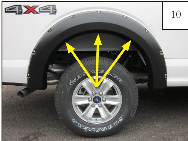
Press flares firmly onto the vehicle and install and fully tighten three screws (SW1-0050) into the clips installed in step 8.
