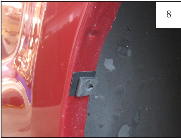
Install a Clip (CL1-0005) over each of the three Tabs (MT1-0014) placed over the upper 3 marks made in Step 6.
