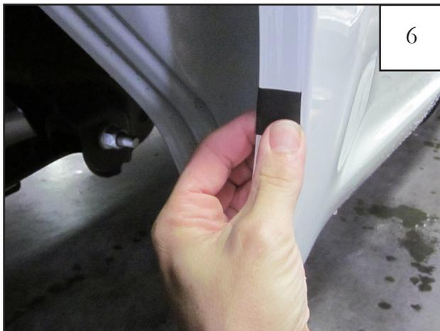
Wrap a Mylar Tab (MT1-0014) around the wheel well sheet metal, centered over each of the three marks made in Step 5.
