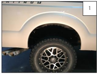
Hold flare to vehicle and ensure that the four holes in flares line up with four factory holes in the fender.
