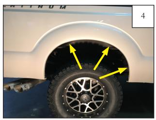
Install "U" clip (CL1-0022) over remaining three tabs.
