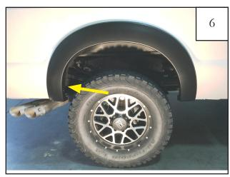
Install a 5/16" Phillips Truss Screw (SW1-0050) into the "S" clip over the rear most hole.
