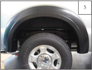
Using a 5/32" Allen Wrench and 3/8" Socket, install bolt, silver washer, spacer, fender washer, and nut through bottom two holes in flare and into factory holes. See step 6.
