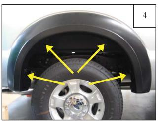
Position flare on fender and, starting with the two top holes, install screws through holes in flare and into clips with a #2 Phillips screwdriver.
