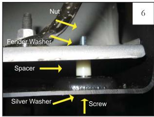
Start bolt from the bottom through a silver washer and into flare. Install spacer between flare and sheet metal. Slide a fender washer then the nut over the end of the screw.
