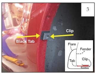
Install a clip over each of the black tabs installed in Step 2.
