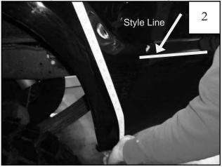
Starting from bottom under edge below mark made in previous step, measure up following curve of wheel well aproximately 15" to lower style line and mark with grease pencil.
