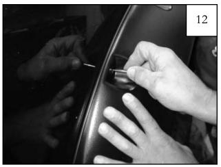
With a partner holding flare in place, using a scratch awl and pocket holes in flare as a guide, mark vehicle for drilling.
