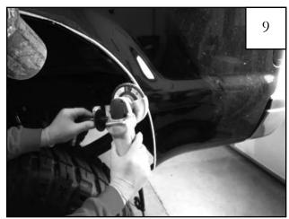
Using a grinder, debur cut edges.
