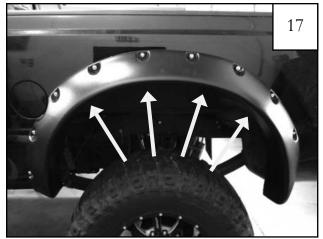
Using a #2 Phillips Driver, fasten screws (SW1-0066) through flare and inter inner fender using holes in flare as a guide.
