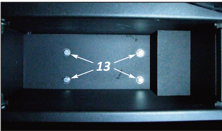
13. Once the stainless steel cage nuts on the lower mounting bracket align with the holes enlarged in Step 11 , install the supplied 1/4-20 x 1-3/4" bolts, 1/4" lock washers and 1/4" flat washers and tighten until the lower mounting bracket secures the console safe to the bottom of the factory console well. Remove any plastic shavings and install the supplied carpet insert into the bottom of the safe.
