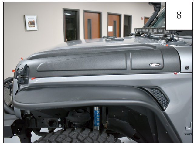
With the Trail Armor in its final position, tack Trail Armor in place by pressing on areas of exposed tape.
