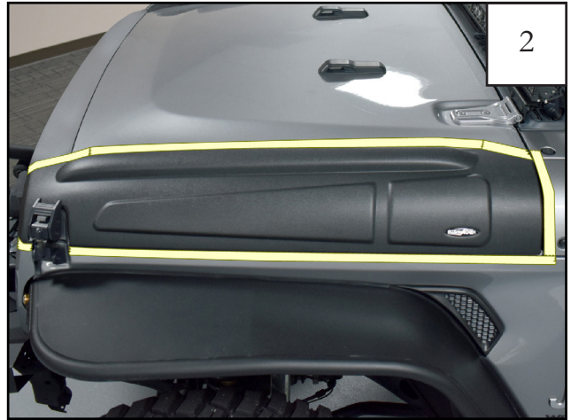
Lay Trail Armor in place on vehicle and mask off the surrounding areas with tape. Remove Trail Armor and set aside.
