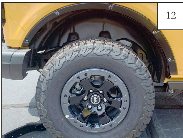
Replace fasteners removed in Step 9 to re-attach fender liner. Completed rear fender delete installation.
