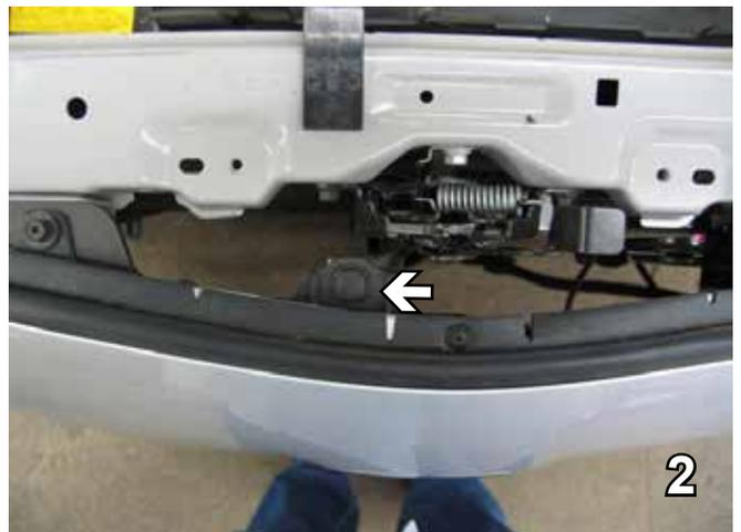
2. Remove push pin from top edge of fascia just below hood latch and set aside for reinstallation later.
