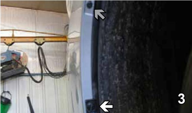
3. Just forward the front tire on the upper corner of the fascia and inside the wheel well, turn the screw 90° to remove it (white arrow). Using a flat screw driver, remove the upper push pin (gray arrow). Do this on both sides and set aside for later reinstallation.
