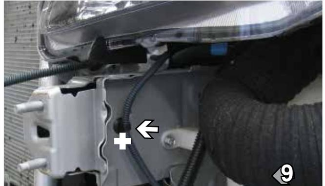
9. On the driver's side pull the wiring out of the existing hole. Drill a hole in the frame rail under but connected with the existing hole using the 1 1/4" hole saw on both sides. This hole will allow the installer to insert the nut plates inside of the frame rail.
