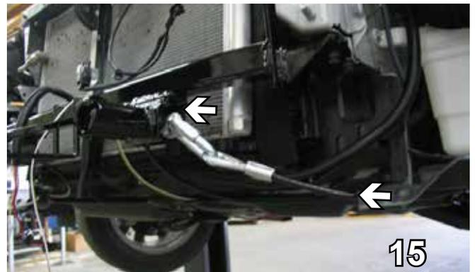
15. Attach baseplate safety cables as in above photos or as close to as possible. If you are unable to place safety cables in this location, position the cables around a solid piece of the frame. Do this on both sides.
