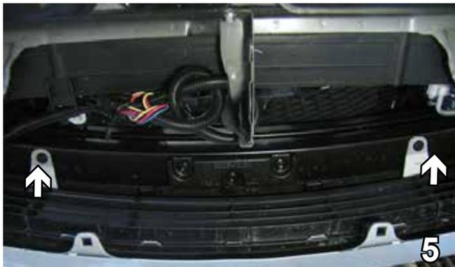
5. Behind the fascia on the bottom of the bumper, are two push pins to remove from the fascia's tabs. Remove with a flat screw driver. Pull the fascia forward on both sides and set aside for later reinstallation.
