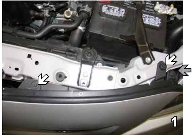
1. Using the Phillips screw driver, remove the Phillips screws (white arrow) from the top corner edge of the fascia. Remove push pin (gray arrow), do this to both sides and set aside for later reinstallation.
