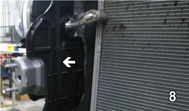
8. Remove the black shield on both sides. It will not be reinstalled.
