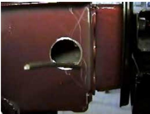
5. Drill 1 1/4" hole on the outside of frame end, just back from seam (see photo for general location), using the 1 1/4" hole saw.
