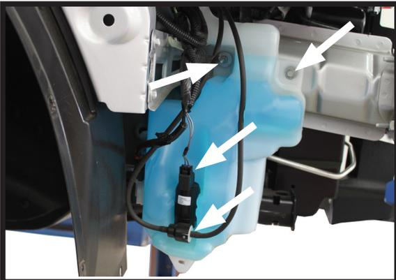
9. The windshield wiper fluid reservoir needs to be removed on the passenger side. Unplug all electrical components and remove the bolt on the top, right side using a 8MM socket. Using a 11MM socket, remove the other two (2) bolts.
