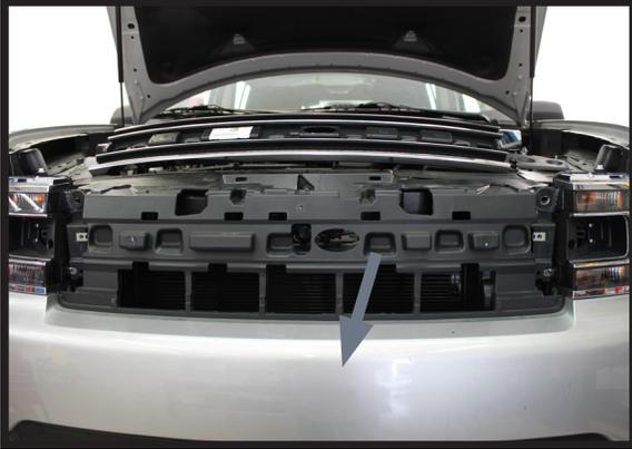
7. The front fascia can now be removed by pulling firmly outward.
