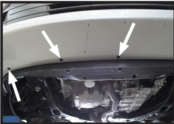
3. On the underside of the vehicle use a 5.5MM socket to remove seven (7) bolts.
