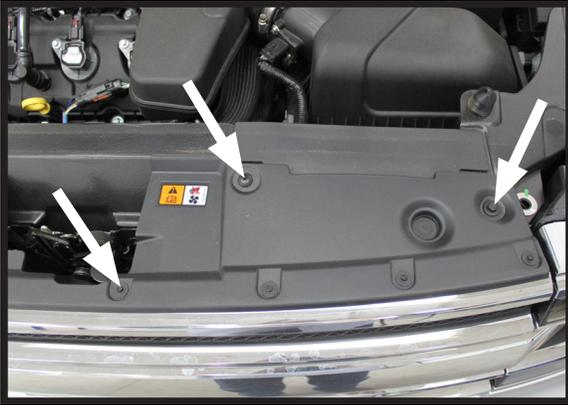
1. Using a 10MM socket, remove the two (2) bolts and push pins that are located in the front area, one (1) per side. There are eight (8) bolts along the front that also need to be removed using a 5.5MM socket.
