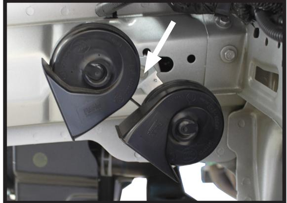
8. On the driver's side, remove the horn using an 8MM socket.
