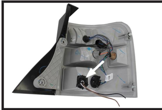
Drill a hole according to the tail
