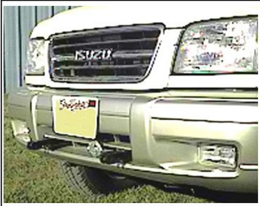
2. Remove the screws located in front of the grill. Pull the grill molding out and set it aside.
