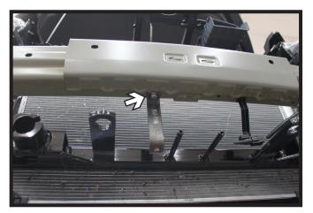
19. **Optional Breakaway:** Attach the breakaway bracket to the bumper in the desired location with the supplied 1/4" hardware. Attach the breakaway to the bracket with the supplied 1/4" hardware.
