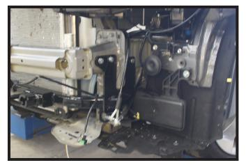
16. Attach the permanent baseplate safety cables to the provided convenience link on the baseplate. The photo above shows the recommended installation of the cables to frame of vehicle. Additional options may interfere with suggested mounting; in this case, secure the cables to a solid piece of the frame as described in the General Information sheet. Be sure the safety cables do not rub against any hoses or moving parts. Do this on **BOTH** sides of the vehicle.
