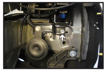
7. Using a 10MM socket, remove the screw from the horn bracket on the driver side and set aside.
