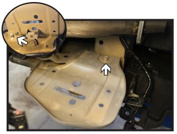
11. Using a 10MM socket, remove the bolt and nut from the metal shielding and set aside. Do this on both sides of the vehicle.
