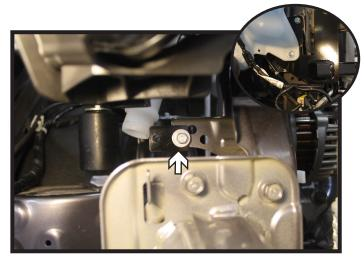
18. Install the washer reservoir bracket onto the upper existing hole with the existing screw. Reinstall the washer reservoir.
