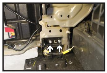
8. Using a 10MM socket, remove the two (2) screws from the sensor bracket and set aside. Do this on both sides of the vehicle.
