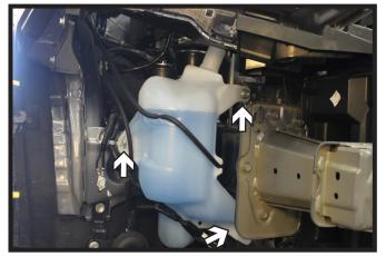
Using a 10MM socket, remove the three (3) screws from the washer reservoir. Disconnect/plug all lines and set aside.
