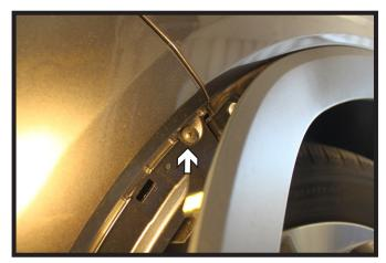
4. Unsnap the fender flare from the fascia. Behind the flare, using a phillips screwdriver, remove the screw from the fascia/fender joint. Do this on both sides of the vehicle.
