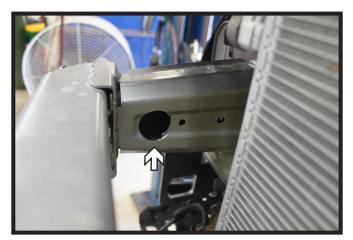
13. On the inside of the passenger side bumper, using a 1-1/2" hole saw, drill an access hole.
