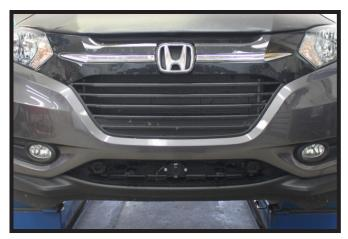
20. Hold the fascia as close to its original position, mark and trim the fascia around the convenience links and attachment tabs. Reinstall the fascia and fascia cover.
