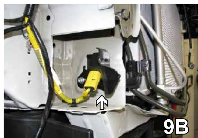
9. Clamp the air bag sensor bracket with the vice grip and bend it back. Do this on both sides.
