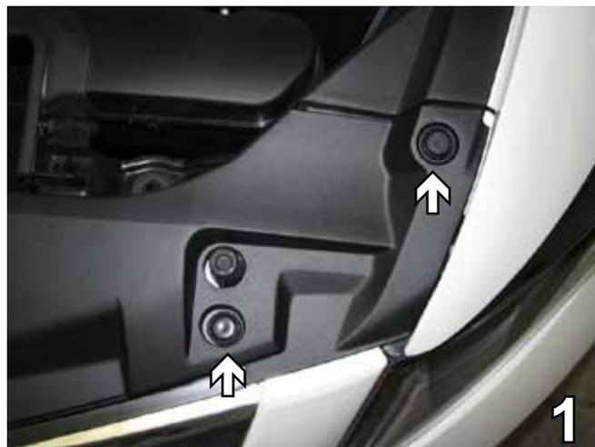
1. Remove two push pins from the side in order to remove the radiator cover. Do this to both sides of the vehicle. Set push pins aside to be reinstalled later.
