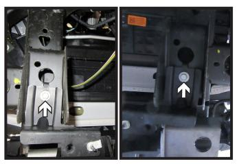
15. Using a 10MM socket, remove the two (2) bolts from the underside of the mounting bracket. Remove bracket and set aside to be reinstalled later.
