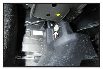
8. Pull back the wheel well liner in front of the tire. Using a 10MM socket, remove the one (1) bolt. Do this on both sides of the vehicle.
