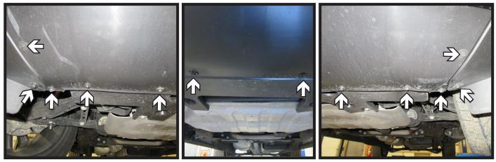
7. Using a 7MM socket, remove the twelve (12) bolts from the side and back of the skid plate.
