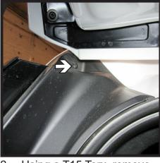
Using a T15 Torx, remove the one (1) bolt at the top of upper plastic cover. Remove upper cover.
