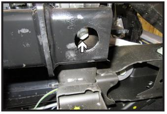
Using a 1/2" drill bit, drill the bottom hole on each side of the baseplate. Then install two (2) 1/2" bolts with lock nuts and whiz nuts, one (1) on each side.
