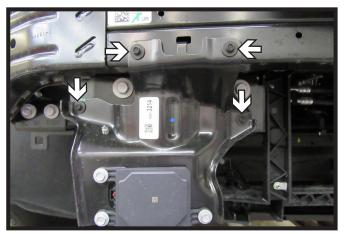
13. **Models with ACC:** Using a 7MM socket, remove the four (4) bolts from the Adaptive Cruise Control (ACC) bracket on the passenger side of the vehicle. Let bracket hang to be reinstalled later.
