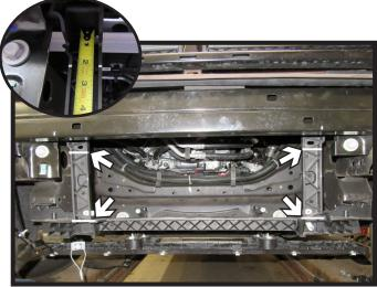
14. Using a saw, cut the two (2) vertical supports of the mounting bracket for the belly pan approximately 2" from the top (inset) and flush with the top of the lower cross member. Remove the cutout pieces.
