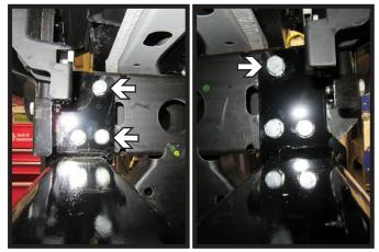
18. Install the remaining three (3) 1/2" bolts with lock washers and whiz nuts into the side holes of the baseplate.
