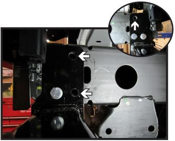
17. Using a 1/2" drill bit, drill the two (2) holes on the passenger side using the baseplate as a template.Note: May need to ream out the top hole
