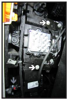
Pull back the wheel well liner. Unplug the electrical on the driver side of the vehicle (gray). Using a 10MM socket, remove the two (2) bolts in front of the tire (white). Do this on both sides of the vehicle.
