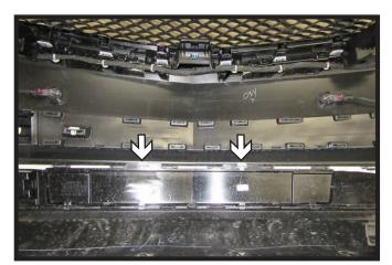
12. On the back side of the fascia, remove the two (2) white clips and pull out center piece from fascia.
