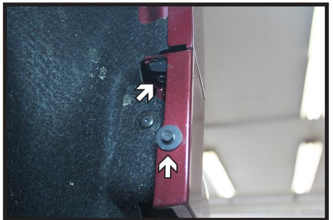
4. Using a 7MM socket, remove the two (2) screws from the wheel well. Do this on both sides of the vehicle. Unsnap the fascia from the body and set aside.
