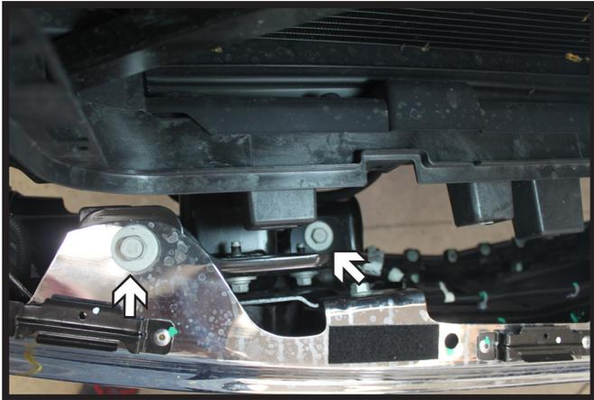
5. Using a 18MM socket, remove the four (4) bolts from the top of the bumper. There are two (2) on each side.
