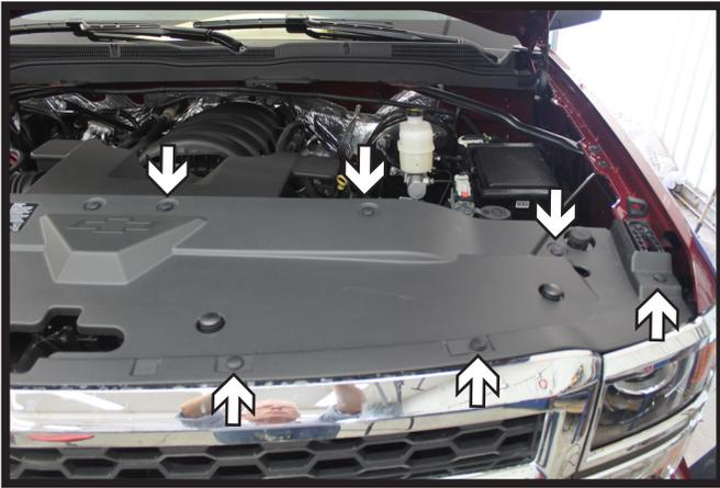
1. Remove the twelve (12) push pins from the fascia cover. There are six (6) on each side. Set the cover aside.
