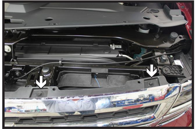
2. Using a 10MM socket, remove the four (4) screws from the top edge of the fascia. There are two (2) on each side.
