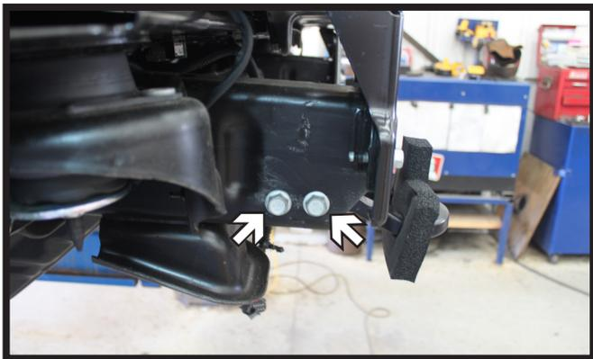
8. Using a 18MM socket/wrench, remove the two (2) bolts from the tow hook. Do this on both sides of the vehicle (left).
