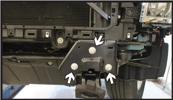
7. Using a 15MM socket, remove the three (3) bolts from the cover plate. Do this on both sides of the vehicle.
