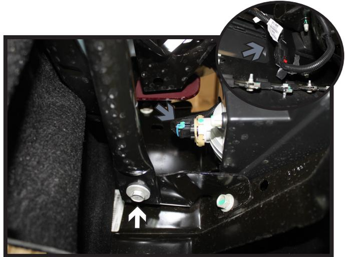
6. Using a 15MM socket, remove the bolt from the bumper reinforcement bar. Do this on both sides of the vehicle. Disconnect the running lights/electrical connections (gray) and set the bumper aside.
