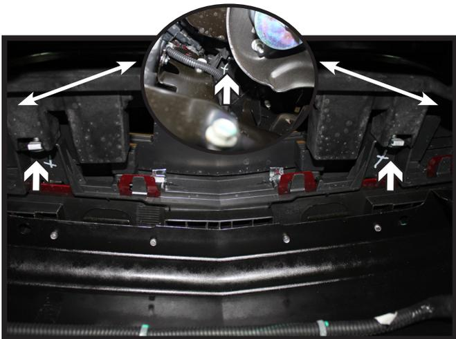
3. Using a 10MM socket, remove the four (4) screws from the underside of the fascia. There are two (2) in the middle and one (1) on each side.
