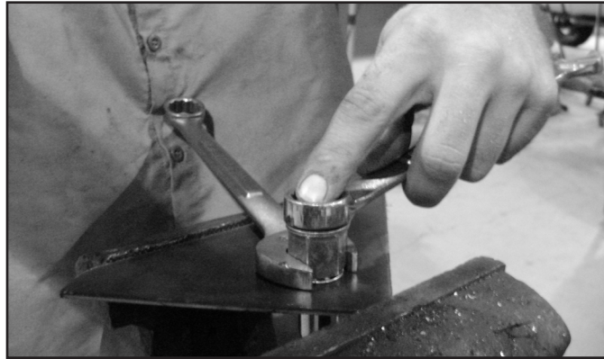
FIGURE 2 - 1/2" RIVET NUT SHOWN
