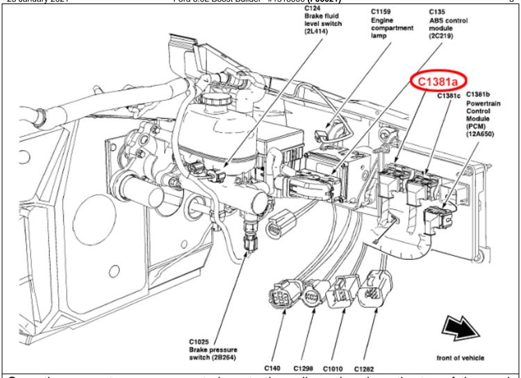
Once the connectors are connected, route the yellow wire along the top of the cowl, over to the driver side. The yellow wire will then connect to the ECM.
