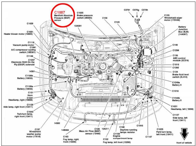
Locate the factory MAP sensor on the passenger side of the vehicle. It should be mounted near the firewall on a pedestal.
