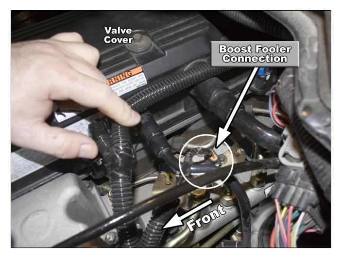
Unplug the factory boost connection from the engine. Plug the BD Boost Fooler inline with the factory plug, and then plug the remaining end of the BD Boost Fooler into the factory plug on the engine.
