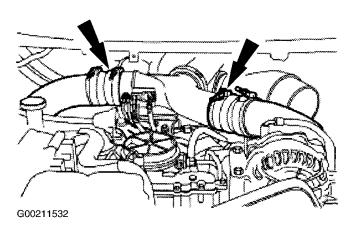
2. Loosen the compressor manifold clamps and remove the compressor manifold. Remove and discard the compressor manifold "O" ring seal.
