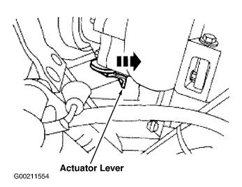
5. On all vehicles, label and disconnect the wastegate actuator vacuum and the pressure lines. Loosen the air inlet tube clamps and remove the air inlet tube.
