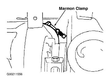
Exhaust inlet Marmon clamp is located behind turbocharger. Loosen the Marmon clamp. Remove the turbocharger retaining bolts and remove the turbocharger. Remove and discard the "O" ring seals.
