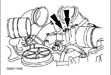
7. Disconnect the exhaust back pressure solenoid electrical connector. Remove the 4 pedestal mounting bolts and remove the turbocharger pedestal. Remove and discard the 2 turbocharger pedestal to engine "O" rings.
