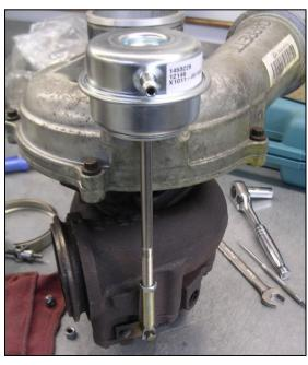
If you would like to adjust the wastegate, loosen the jam nut and slide the rod end off of the wastegate lever shaft. Turn the rod end in or out depending on how you want to adjust the boost pressure.
