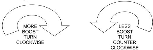
To increase the boost pressure you will have sufficient energy to drive the turbo faster. Once you have turned the rod to the desired position, re-install the circlip and lock the jam nut.
