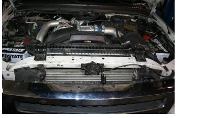
12. Mount the (1407008) 3-3 1/4" step ribbed boots on the BD intercooler and tighten the (1407030) 3 1/2" clamps until the spring is bound. (1/2" head)
