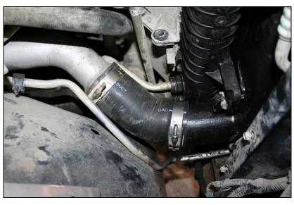
You will need two people for this part to avoid damaging any fins. Pull the condenser and transmission cooler forward, lift the radiator up out of the grommets on the CAC and push it back, then carefully remove the CAC.
