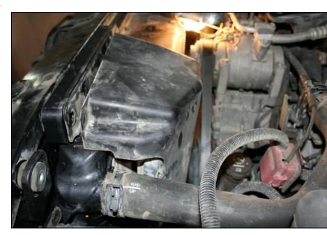
With a 10mm socket, install the hood latch with the 3 bolts taken off earlier (The position is critical, make sure it lines up to the tie bar paint pen marks).
