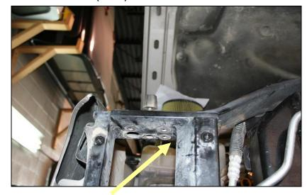
Remove the upper tie bar with a 10mm socket. There are 3 on each end coming up from the bottom and 2 on each side on the lower struts.
