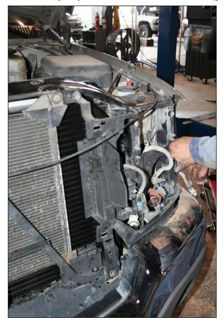
Install the grille by pushing all the clips into the receivers and the 1 bolt in holding the grille to the upper tie bar with a 10mm socket.
