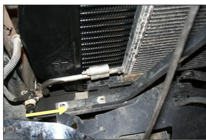
Loosen the boot clamps with a 7/16 deep socket on both the driver's and passenger side.
