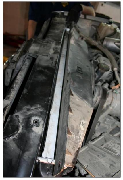
Remove the 2 brackets that secure the bottom of the radiator to the CAC. Unbolt the radiator from the CAC, followed by the 2 bolts that secure the CAC to the upper tie bar with a 13mm socket.
