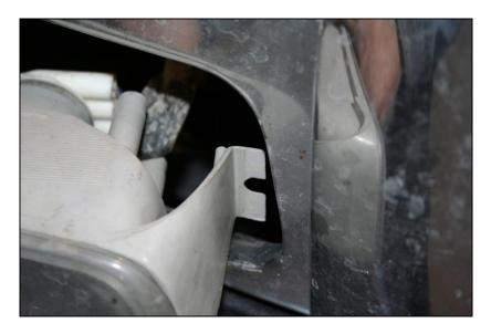
Install the marker lights by tucking in the inside tab first, and then push the outer clip into the headlight panel.
