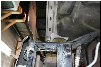
Install the upper tie bar with a 10mm socket. There are 3 on each end coming up from the bottom and 2 on each side on the lower struts.
