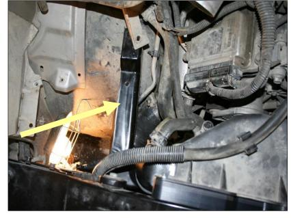
With a 10mm socket, remove the three hood latch bolts (The position is critical, mark where it lines up to the tie bar with a paint pen).
