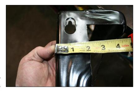
The bracket that supports the air box will need to be modified as shown, and then painted for corrosion resistance.
