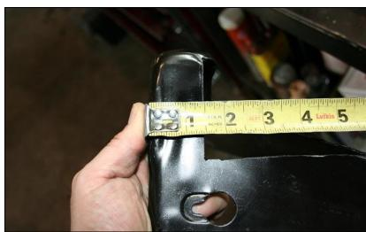
Install the metal support bracket onto the loosened bolts still in the radiator support, tighten them and install the one that holds the coolant reservoir to the bracket with a 10mm socket.
