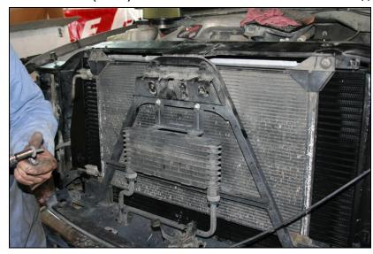
Install the driver's side support strut to the tie bar with a 10mm socket.
