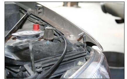
Remove the headlights by pulling the mounting pins to detach them from the mounting panel.
