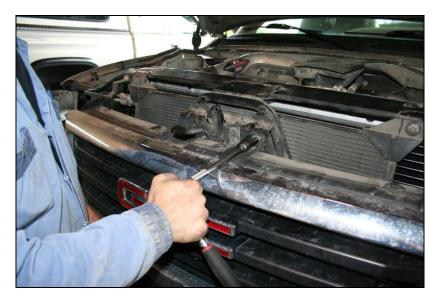
Remove the 1 bolt holding the grille to the upper tie bar with a 10mm socket. Use a clip removal or similar tool to release these clips shown here, and the far outer clips can be removed by pulling them out by hand.
