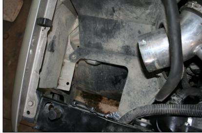
Under your air box there is a metal support bracket to remove. Loosen it but do not remove the two 10mm bolts that hold it to the radiator support. Remove one that holds the coolant reservoir to the bracket.
