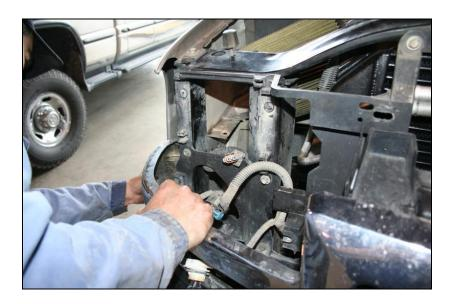
Remove the two headlight mounting panels. There are 6 - 10mm and 2 - T25 Torx.
