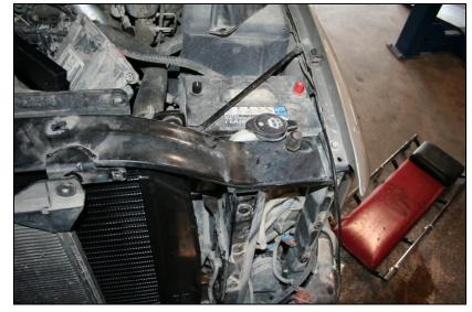
While you can still clearly see the hood latch, bring down the hood to make sure the latch will line up, and if it does, do a test by closing it before continuing.
