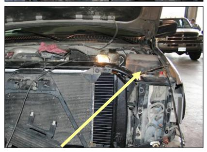
Remove the upper fan shroud. There are 2 push fasteners on each side holding it to the lower shroud and 4 - 10mm head bolts across the top to the tie bar.
