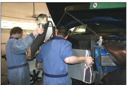
When installing the intercooler, ensure that none of the transmission lines or A/C condenser lines is rubbing on the front vehicle supports.
