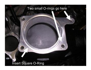
Flip the BD Intake over and insert the intake over and down through the studs until it is mounted to the factory intake plenum.
