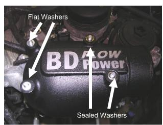
Insert the 4 M6 Acorn nuts onto the studs and torque to 8 ft-lbs (96 in-lbs).
