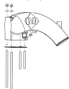
Reuse the factory dipstick tube mounting bolt to secure the dipstick to the intake.
