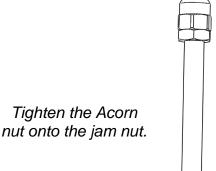
Note that the end with the shorter length of thread, should be inserted into the head.
