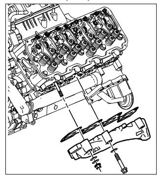
Use the sequence shown to properly tighten the exhaust manifold bolts.
