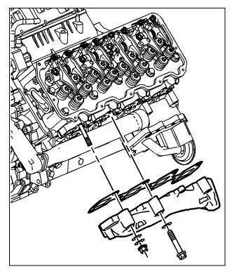
With the stock heat shield removed, reform the heat shield to the new BD high flow exhaust manifold on a clean bench. Allowing clearance around the new manifold.
