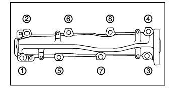
Remove the exhaust manifold.
