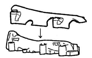
Install the BD High Flow exhaust manifold with gasket.
