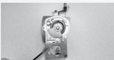
Using the puller tool remove the motor.
