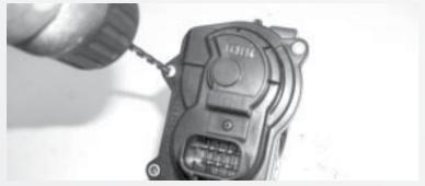
Using a drill with a 3/16 bit CAREFULLY drill out the rivets that attach the throttle body motor housing to the throttle body.
