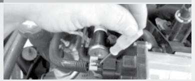
Unplug the throttle body electric motor by removing the gray colored locking clip, and then squeezing the tab on the wiring connector while pulling it from the motor housing.
