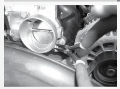
Using pliers remove the coolant pass through hoses from the bottom of the throttle body by squeezing the tabs on the hose clamps together and pulling the hoses away from the throttle body.
