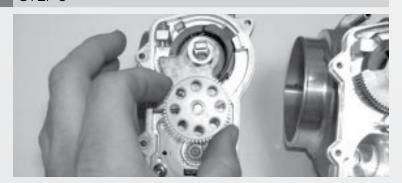
Remove the round idler gear from the throttle body.
