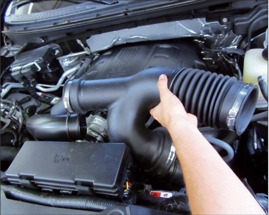
**6.** Un-latch 3 clips holding OEM lid, to air filter housing. See **Figure 6**.
