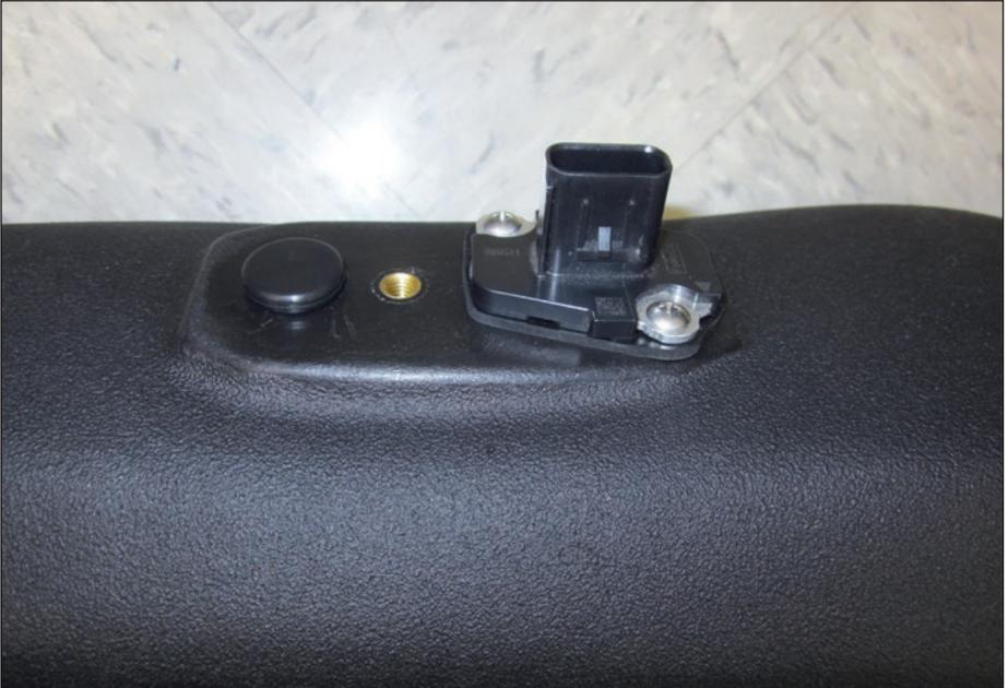
(41872) using the two provided 6-32 screws (91719). Install the Map Sensor Plug (41876) into the adjacent sensor port.
