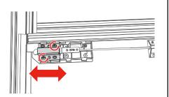
With the latch cover removed, loosen the screws and move the latch bracket to adjust. Retighten the screws. Slide the latch housing back on.
