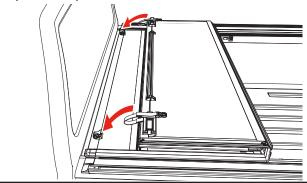
**FLIPPED UP POSITION**: Fold the cover (A) open and lift it until it's vertical or past 90 degrees towards the truck cab. Then release the prop rod that is attached to the rail. Fold the prop rod over and position it firmly against the vertical plate on the underside of the cover. Then slide the prop rod locks downwards and tighten the
