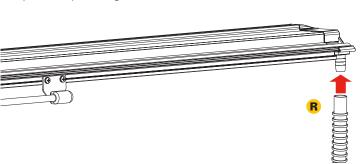
Place the driver side rail (B) on the truck rail. Position the side rail flush with the top edge of your truck bed rail. The end of the side rail with the drain tube will go towards the cab of the truck. Repeat on the opposite side with the passenger side rail (C).
