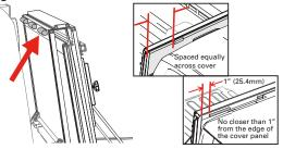
Unfold the cover (A) towards the tailgate. Then confirm each panel is centered side to side and front to back on the truck bed. If adjustments are needed, loosen the cover retainer clamps (G) and shift the cover until positioned correctly. The rear edge of the cover and tailgate seal should rest on top of the tailgate. For proper sealing, the tail panel will overlap by .5".
