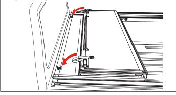
FLIPPED UP POSITION: Fold the cover (A) open and lift it until it's vertical or past 90 degrees towards the truck cab. Then release the prop rod that is attached to the rail. Fold the prop rod over and position it firmly against the vertical plate on the underside of the cover. Then slide the prop rod locks downwards and tighten the knobs to lock it into position. Do this on both sides of the cover. The cover should be firmly in position with little to no movement once the prop rods are locked.
