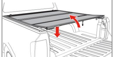
**FOLDED UP POSITION:** To drive with the cover (A) in the folded up position, use the straps and buckles provided with the cover. Attach the buckle at the bulkhead, then pull the strap to take up the slack and secure the cover.
