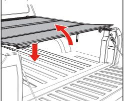
**FOLDED UP POSITION:** To drive with the cover (A) in the folded up position, use the straps and buckles provided with the cover. Attach the buckle at the bulkhead, then pull the strap to take up the slack and secure the cover.
