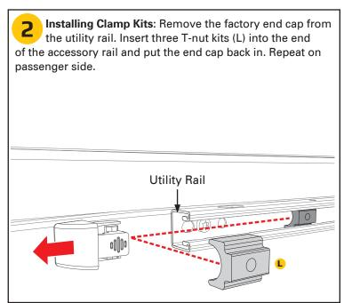
Installing Adapter Rail: Install adapter rail driver side (D) with the bolt, washer and lock washer that is attached to the T-nut kit (L) and push the rail all the way toward the cab and the bulkhead. Adjust the t-nuts so they are lined up with the holes in the adapter rail. Leave loose at this time. Repeat on passenger side.
