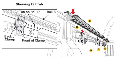
**NOTE**: If the rails are leaning down, have one person stand on the outside of the bed and slightly roll the rails upward while another person slowly snugs the clamps up. If the clamps are tightened too quickly or overtightened, it will cause the rails to lean down.
