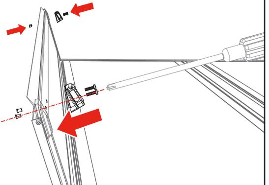
**9** Set the cover (C) in the folded position on the side rails (A & B) towards the cab of the truck. Confirm the cover is evenly spaced between the rails.
