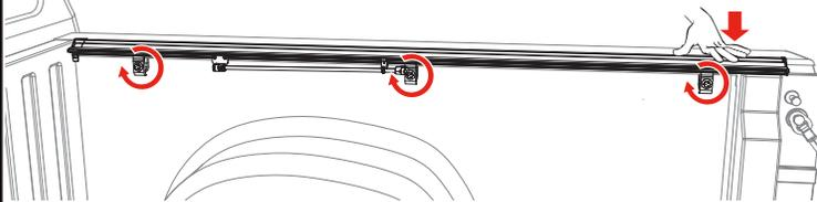
**NOTE:** If the rails are leaning down, have one person stand on the outside of the bed and slightly roll the rails upward while another person slowly snugs the clamps up. If the clamps are tightened too quickly or overtightened, it will cause the rails to lean down.
