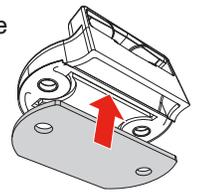
Position the buckle ends (H) with the open side facing the bed cover panel. Use a Phillips screwdriver to install the two buckles into the pre-drilled holes on the front header panel with the provided screws (I) and the nutsert (J) inserted from the backside of the panel. **DO NOT use a screw gun, securely tighten by hand only.**
