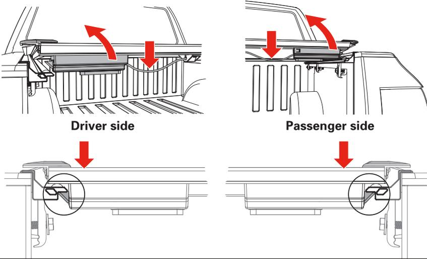
**14** Retighten the cover retainer clamps (F) once the desired fitment is reached. **You are ready to drive with your cover in the closed position.**
