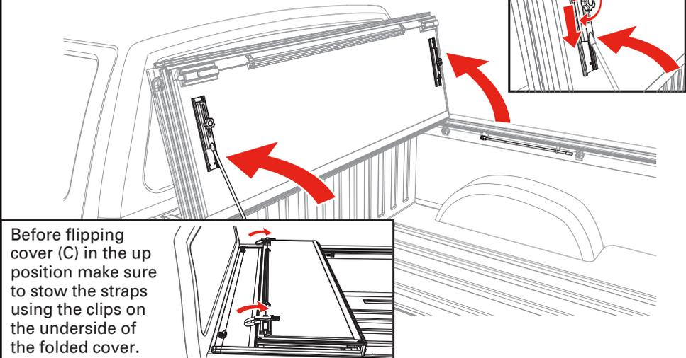
**CLOSING COVER:** To drive with the cover (C) closed, unhook the buckles and straps from the bulkhead. Stow the straps using the clips on the underside of the folded cover. Fold all panels towards the tailgate making sure that all latches are engaged.
