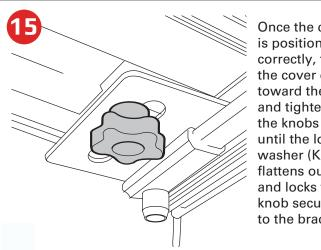
Once the cover is positioned correctly, fold the cover over toward the cab and tighten the knobs (L) until the lock washer (K) flattens out and locks the knob securely to the bracket.
