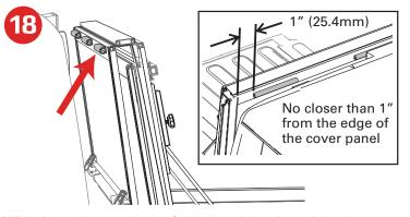
With the bed cover in the folded position, install the three D-shaped cab bumpers (E) along the top edge of the cover where it meets the truck cab.
