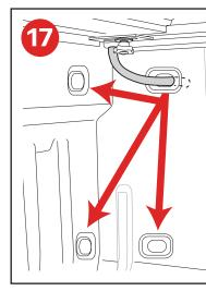
Route the other end of the drain tube (F) through the factory bed plug. Simply remove these plugs or drill a 7/8" hole through the plastic. Alternately, the plug can be trimmed using a utility knife making sure to cut a hole large enough to not crimp the drain tube.NOTE: If you have a drop-in bedliner, simply run the drain tubes behind or under the liner.
