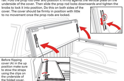
**CLOSING COVER:** To drive with the cover (A) closed, unhook the buckles and straps from the bulkhead. Stow the straps using the clips on the underside of the folded cover. Fold all panels towards the tailgate making sure that all latches are engaged.
