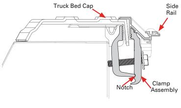
Attach one stake pocket clamp (U) from the passenger side rail (A) to the truck bed. Disassemble the stake pocket clamp (U). Place the inner part of the clamp into the rail. Make sure the bolt passes through the stake pocket hole as shown.
