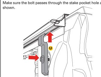
Place the outer part of the stake pocket clamp (U) into the stake pocket, up underneath the plastic bed cap, then secure to the bolt. Make sure the rail is level. Tighten all clamps to 10 ft/lbs of torque with a 1/2" wrench or socket. Caution: Do NOT overtighten! Note: For 07-13 models only, install stake pocket covers (V) into stake pocket opening in the side rail toward tail. Repeat for driver's side rail (B).
