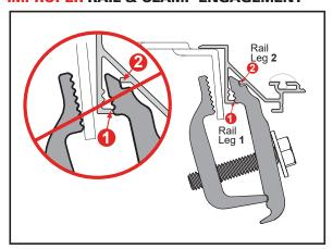
Water Intrusion: Make sure the retaining clamps are tight and properly engaged to the side rails. Check that the bulkhead seal is in place and the cover is resting on it. Make sure that all latches are engaged to the side rails and adjust if needed. Check that the side rails are installed flush with the top of the bed rail.
