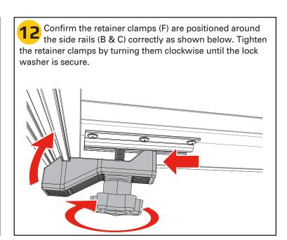
Confirm the retainer clamps (F) are positioned around the side rails (B & C) correctly as shown below. Tighten the retainer clamps by turning them clockwise until the lock washer is secure.
