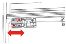
With the latch cover removed, loosen the screws and move the latch bracket to adjust.
