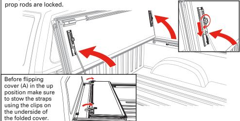
**CLOSING COVER:** To drive with the cover (A) closed, unhook the buckles and straps from the bulkhead. Stow the straps using the clips on the underside of the folded cover. Fold all panels towards the tailgate making sure that all latches are engaged.
