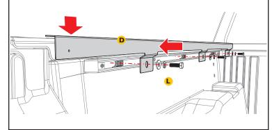
When you get the adapter rail driver side (D) and the T-nut kits (L) lined up you can now tighten the bolts while you are applying downward pressure to the rail. A second set of hands may help. Repeat on the opposite side using the adapter rail passenger side (E).
