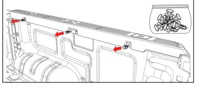
Attach the drain tubes (O) to the front of the side rails (B & C) to allow water to be diverted out of the truck bed via the rail. The opposite end of the drain tubes can be placed behind a bedliner, through the bed plugs, or by drilling a 5/8" hole in the bulkhead.
