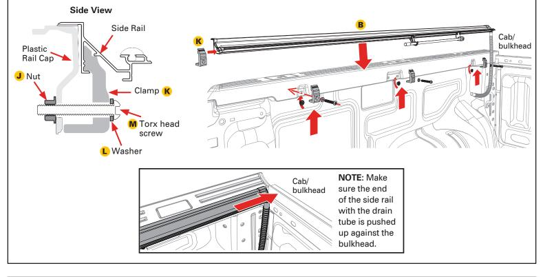
Starting with the front clamp, make sure the rail (B) is pushed forward against the bulkhead, and square with the bed rail, apply downward pressure on the rail while tightening the Torx head screw with a T-30 Torx bit to 8ft.lbf/11N.m. and a 1/2" wrench on the nut. Repeat with the middle and then rear clamp, making sure the rail is square and flat with the bed rail. Caution: Do NOT overtighten. Repeat on passenger side rail (C).
