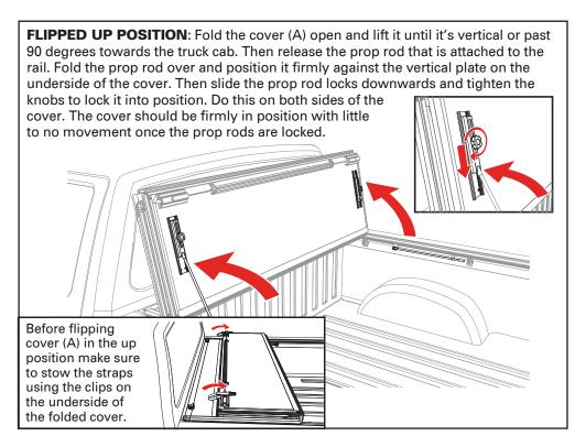
**OPENING COVER:** Lower the tailgate and pull the cable on either side. While pulling on the cable lift the panel up
