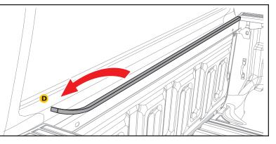
If rubber filler strips (E) were NOT included in your kit, skip to step 3. If you received rubber filler strips (E) with the cover (C), clean the rail the same way as you did in step 1. Peel the backing and adhere the filler strips (E), as illustrated, between the truck plastic bed cap and truck metal rail. Place one 6-8 inches from the bulkhead. Place the rear strip as close to the tailgate as possible. Center the middle strip appropriately.
