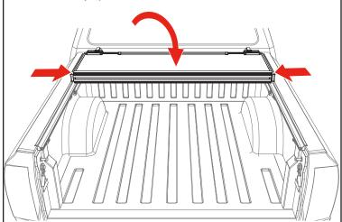
Confirm the retainer clamps (E) are positioned around the side rails (B & C) correctly as shown below. Tighten the retainer clamps by turning them clockwise until the lock washer is secure.
