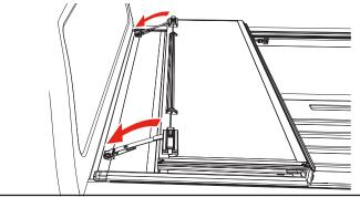
**FLIPPED UP POSITION:** Fold the cover (A) open and lift it until it's vertical or past 90 degrees towards the truck cab. Then release the prop rod that is attached to the rail. Fold the prop rod over and position it firmly against the vertical plate on the underside of the cover. Then slide the prop rod locks downwards and tighten the knobs to lock it into position. Do this on both sides of the cover. The cover should be firmly in position.
