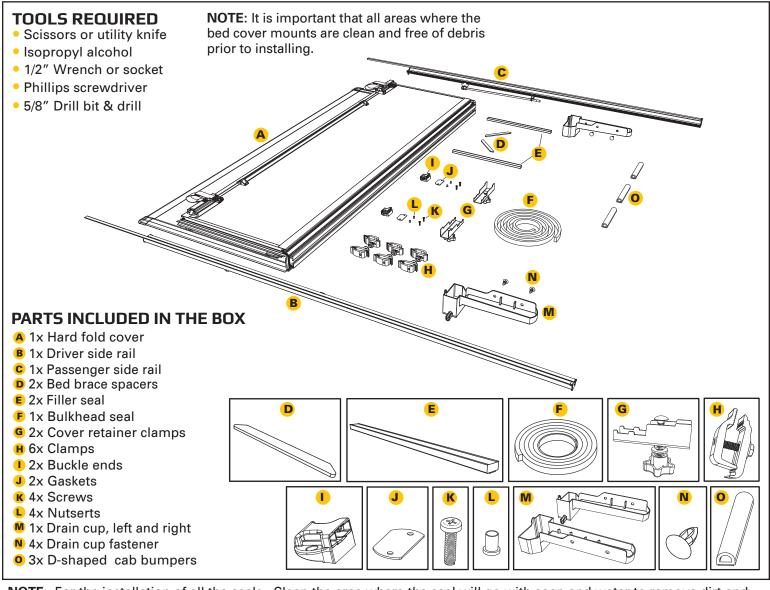
**NOTE**: For the installation of all the seals. Clean the area where the seal will go with soap and water to remove dirt and debris. Then clean the area with isopropyl alcohol to remove wax or grease and to evaporate any remaining water. Allow the surface to dry.
