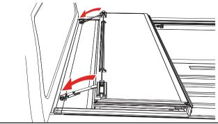
**FLIPPED UP POSITION:** Fold the cover (A) open and lift it until it's vertical or past 90 degrees towards the truck cab. Then release the prop rod that is attached to the rail. Fold the prop rod over and position it firmly against the vertical plate on the underside of the cover. Then slide the prop rod locks downwards and tighten the knobs to lock it into position. Do this on both sides of the cover. The cover should be firmly in position with little
