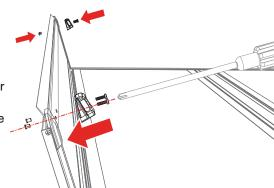
Set the cover (A) in the folded position on the side rails (B & C) towards the cab of the truck. Confirm the cover is evenly spaced between the rails.
