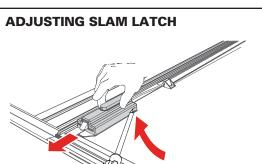
Use a screwdriver to partially pry open the tab on the latch housing. At the same time slide the housing away from the latch assembly.
