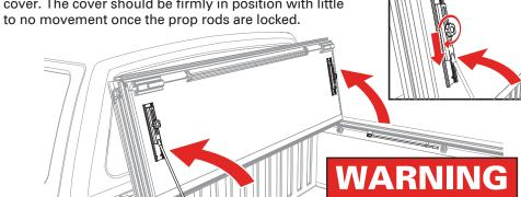
CLOSING COVER: To drive with the cover (A) closed, unhook the buckles and straps from the bulkhead. Stow the straps using the clips on the underside of the folded cover. Fold all panels towards the tailgate making sure that all latches are engaged.
