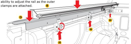
**NOTE:** If the rails are leaning down, have one person stand on the outside of the bed and slightly roll the rails upward while another person slowly snugs the clamps up. If the clamps are tightened too quickly or overtightened, it will cause the rails to lean down.
