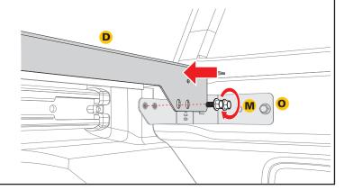
Install the adaptor rail driver side (D) by lining up the studs with the holes in the rear bracket using two M6 flange mounting bolts (M) and two 1/4-20 nuts (N). Repeat on the opposite side using the passenger side adaptor rail (E). Now tighten, using a 7/16" socket in front and rear on both sides.
