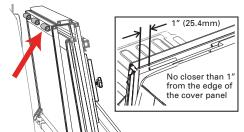
Unfold the cover (A) towards the tailgate. Then confirm each panel is centered side to side and front to back on the truck bed. If adjustments are needed, loosen the cover retainer clamps (G) and shift the cover until positioned correctly. The rear edge of the cover and tailgate seal should rest on top of the tailgate. For proper sealing, the tail panel will overlap by .5".
