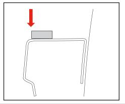
Attach the drain tubes (K) to the front of the side rails (A & B) to allow water to be diverted out of the truck bed via the rail. The opposite end of the drain tubes can be placed behind a bedliner, through the bed plugs, or by drilling a 5/8" hole in the bulkhead.
