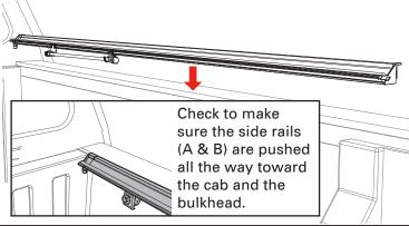
Attach three clamps (F) to the driver side rail (B) to the truck bed. Place the front clamp 6-8 inches from the bulkhead. Place the rear clamp as close to the tailgate as possible. Center the middle clamp accordingly. Clamps should be evenly spaced along the full length of the rail. Loosely tighten with a 1/2" wrench to make sure the clamps engage with the side rail.
