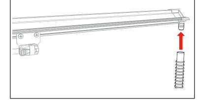
Place the passenger side rail (A) on to the passenger side mounting rail (N) installed in the previous steps. Position the side rail flush with the top edge of the mounting rail. The end of the side rail with the drain tube goes toward the cab of the truck.
