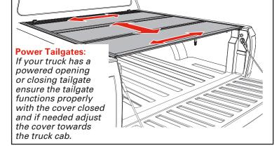
Check if the latches are hitting or not engaging the side rails (B & C) by releasing each latch. If any of the latches need modifications refer to the Slam Latch Adjustment section on the next page on how to make adjustments.
