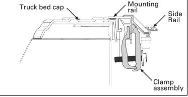
Before placing the cover (C) onto the vehicle, slide two cover retainer clamps (E) into the track on the underside of the cover near the cab. Confirm the cover retainer clamps fit properly into the cover rail for optimum fit. Repeat on the opposite side of the cover.
