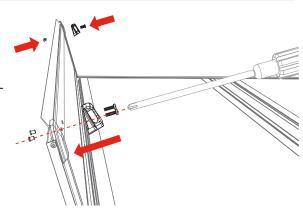
Set the cover (C) in the folded position on the side rails (A & B) towards the cab of the truck. Confirm the cover is evenly spaced between the rails.
