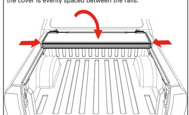
Confirm the retainer clamps (E) are positioned around the side rails (A & B) correctly as shown below.
