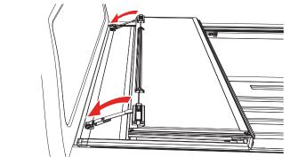
FLIPPED UP POSITION: Fold the cover (A) open and lift it until it's vertical or past 90 degrees towards the truck cab. Then release the prop rod that is attached to the rail. Fold the prop rod over and position it firmly against the vertical plate on the underside of the cover. Then slide the prop rod locks downwards and tighten the knobs to lock it into position. Do this on both sides of the cover. The cover should be firmly in position with little to no movement once the prop rods are locked.
