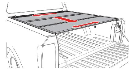
Check if the latches are hitting or not engaging the side rails (B & C) by releasing each latch. If any of the latches need modifications refer to the Slam Latch Adjustment section on the next page on how to make adjustments.
