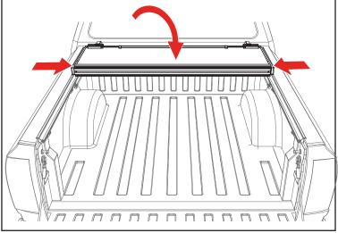
Confirm the retainer clamps (E) are positioned around the side rails (B & C) correctly as shown below. Tighten the retainer clamps by turning them clockwise until the lock washer is secure.
