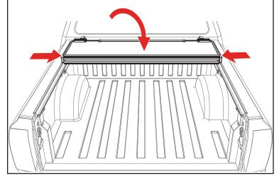
**10** Confirm the retainer clamps (E) are positioned around the side rails (B & C) correctly as shown below. Tighten the retainer clamps by turning them clockwise until the lock washer is secure.
