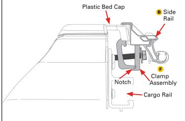
3 Slide three front halves of the clamp (F) into the rail in the tapered slot. Position the rear front half of the clamp (F) as close to the tailgate as possible. It should be less than 12". Place the second front half of the clamp (F) near the center of the rail. Position the third front half of the clamp (F) as close to the front of the rail as possible. It should be less than 12" from the front.
