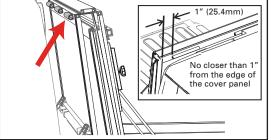
Unfold the cover (A) towards the tailgate. Then confirm each panel is centered side to side and front to back on the truck bed. If adjustments are needed, loosen the cover retainer clamps (E) and shift the cover until positioned correctly. The rear edge of the cover and tailgate seal should rest on top of the tailgate. For proper sealing, the tail panel will overlap by .5".
