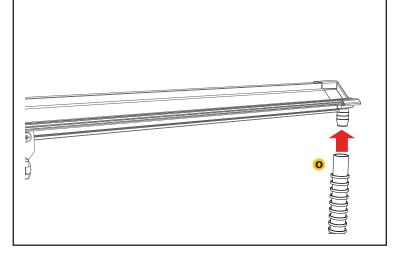
Route the other end of the drain tube (O) through the tie-down hook and into the factory bed plug. Remove this plug first or drill a 7/8" hole through the plug. Alternately, the plug can be cut using a utility knife, making sure to cut a hole large enough to not crimp the drain tube. NOTE: If you have a drop-in bedliner, just route the drain tubes behind the liner. Repeat on the driver's side.
