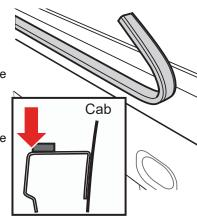
off, exposing the top of the front bulkhead. Place the front bulkhead seal as previously instructed. This will allow the front bulkhead seal to sit flush with the top of the bed caps.
