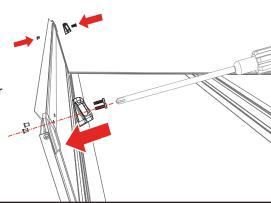
Set the cover (A) in the folded position on the side rails (B & C) towards the cab of the truck. Confirm the cover is evenly spaced between the rails.
