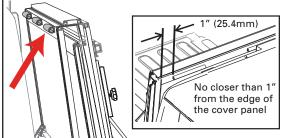
Clean the tailgate extrusion of the hard fold cover (A). Then peel the backing from the tailgate seal (P) and adhere the seal from one tailgate extrusion edge to the other. Apply pressure evenly to the entire seal to ensure proper adhesion.
