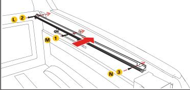
Clean the area where the plate (G) will go with soap and water to remove dirt and debris. Then clean the same area with isopropyl alcohol to remove wax or grease and to evaporate any remaining water. Allow the surface to dry. Peel the two backing strips from the plate and center over recessed area. Apply pressure to the entire plate to make sure adhesion is good. Repeat on driver's side rail (B).
