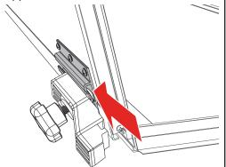
First, prep the buckle ends (H) by peeling off the adhesive liner of the gasket (I).
