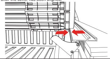
When correctly installed, the vinyl edges of the cover (E) will align squarely with the side rails in all four corners. The latch assembly will align with the side rail locking levers at the tailgate on both sides.
