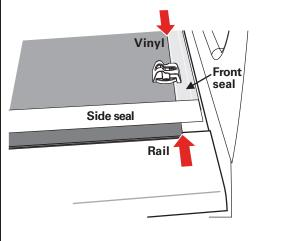
Verify that a gap of approximately 1/8" (3.2mm) remains on both sides of the cover (E) between the edge of the cover rail and the rolling cover. This spacing is necessary to ensure that the locking rail secures to cover. Align the cover side to side at the front and/or the back if the side gaps are not even. Firmly hand tighten the knobs (H) after the cover has been aligned.
