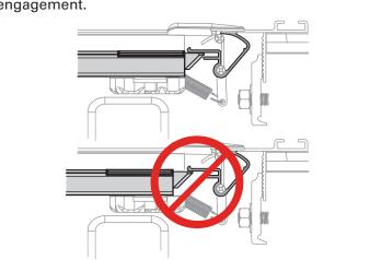
When the cover (E) is properly aligned, roll the cover open, ensuring not to misalign while opening.
