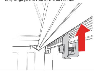
Mount the strap clamp assembly (F) as far forward as possible. Hand tighten to 10 ft/lbs of torque with
