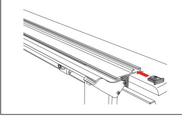
**ROLLED UP POSITION:** To drive with the cover (E) in the open position, use the strap clamps. Roll the cover forward, twist and insert the clips into the cover clasps. Ensure that BOTH strap clamps are fully inserted into the clasps. Pull on the end of the strap to tighten.
