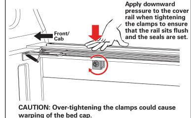
**NOTE:** When installing each clamp (G), make sure that the clamps are inserted as far up onto the rail as possible and that the clamp teeth fit squarely and fully engage the ribs of the cover rail.
