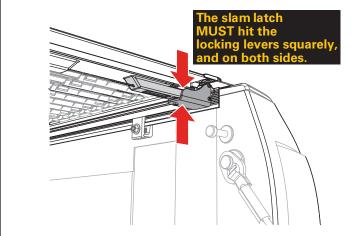
Check to see that the latches on both sides at the tailgate fully engage the cover rails (A & B). Loosening the knobs (H) and making the side to side adjustment as in step 18 could help with the latch striker engagement.
