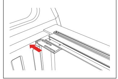
Start at the front and place the first clamp (G) onto the rail, approximately 6 to 9 inches back. Make sure the cover rail is clamped square and level. Hand tighten to 10 ft/lbs of torque with a 9/16" wrench or socket.
