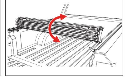
Align the front vinyl edge of the rolled cover (E) with the front edge of the side rails (not the rubber seal).
