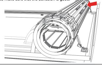
Install one end cap (C) on the rearward portion ONLY of the new passenger side cover rail (A), as shown. Tighten the set screw with the provided Allen wrench. Do this also on the new driver side cover rail (B).
