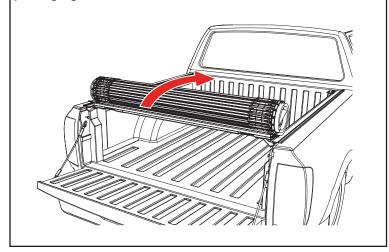
Fold the front panel back and insert the two mounting bolts (K) into the slotted bracket. Do this for both sides. The bolts will align with the slotted bracket of the cover rail. Fold the panel back down.
