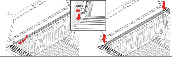
Position the new passenger side cover rail (A) on the truck rail with the slotted bracket pushed all the way toward the front/cab and the bulkhead.
