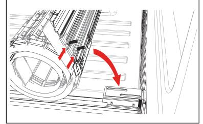
Install the mounting hardware from step 2 loosely underneath the slotted bracket on the passenger cover rail (A). Start with the rubber washer (J), then the large flat washer (I), then hand tighten the lock knobs (H). Repeat on the driver's side. Leave the knobs loose for now.
