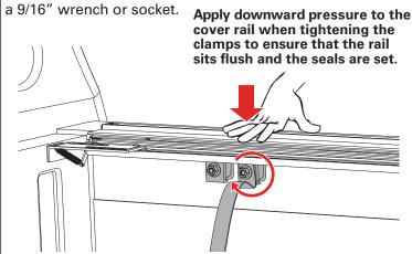
CAUTION: Over-tightening the clamps could cause warping of the bed cap.
