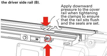
**CAUTION**: Over-tightening the clamps could cause warping of the bed cap.
