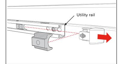
Install a strap clamp (L) to the passenger side adaptor rail (E) near the front/cab with a T-nut kit (N) (a bolt, lock washer, washer and t-nut). Position the passenger side adaptor rail (E) about a half an inch from the front/cab. Adjust the t-nut so it is lined up with the hole in the adaptor rail. Leave loose at this time.
