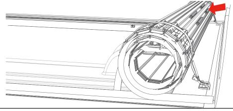
If the side seals of the cover appear wrinkled, exposure to the sun will assist the seals to lay flat. Applying heat with a hair dryer or carefully with a heat gun will also smooth the seals.
