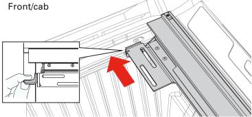
**NOTE**: Some drop-in bed liners may require trimming in the corners to fit the rail into the opening.
