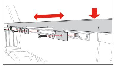
After you get the adaptor rail and the T-nut kits lined up, you can now tighten the bolts, while you are applying downward pressure to the rail (E). Tighten to 10 ft/lbs of torque with a 1/2" wrench or socket. A second set of hands may help. Repeat on the opposite side with the passenger side adaptor rail (F).
