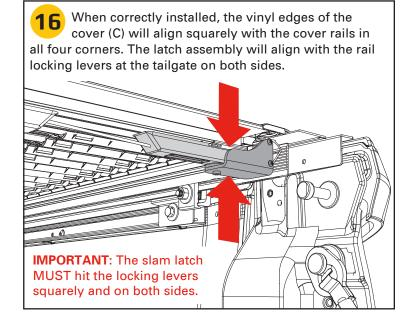
Check to see that the latches on both sides at the tailgate fully engage the cover rails. Loosening the knobs (H) and making the side to side adjustment as in step 8 could help with the latch striker engagement.
