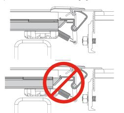
When the cover (C) is properly aligned, roll it open, ensuring not to misalign while opening, and tighten the knobs (H) on both sides to secure the cover. DO NOT overtighten. Hand tighten only. Recheck that the cover operates correctly. Close the cover and check that the locking levers are engaged and prevent the cover from being lifted on both sides.
