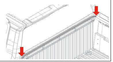
Position the passenger side cover rail (A) on the adaptor rail with the slotted bracket pushed all the way toward the front/cab and touching the cargo rail. If the truck is equipped with a drop-in bedliner, remove the foam pads located at the front of the slotted brackets.
