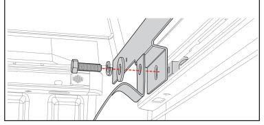
Install the rest of the adaptor rail (E) with the T-nut kits (N). Adjust the t-nuts so they are lined up with the holes in the adaptor rail. Leave loose at this time. Repeat steps 9-10 on the driver side with the driver side adaptor rail (F).
