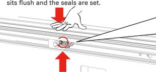
**CAUTION**: Over-tightening the clamps could cause warping of the bed cap.
