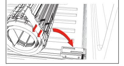
Install the mounting hardware loosely underneath the slotted bracket on the passenger cover rail (A). Start with the rubber washers (J), then the large flat washers (I), then hand tighten the knobs (H). Repeat on the driver side. Leave the knobs loose for now.
