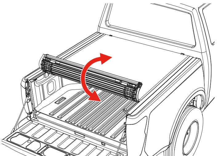
**10** Align the front vinyl edge of the rolled cover (C) with the front edge of the cover rails (not the rubber seal).
