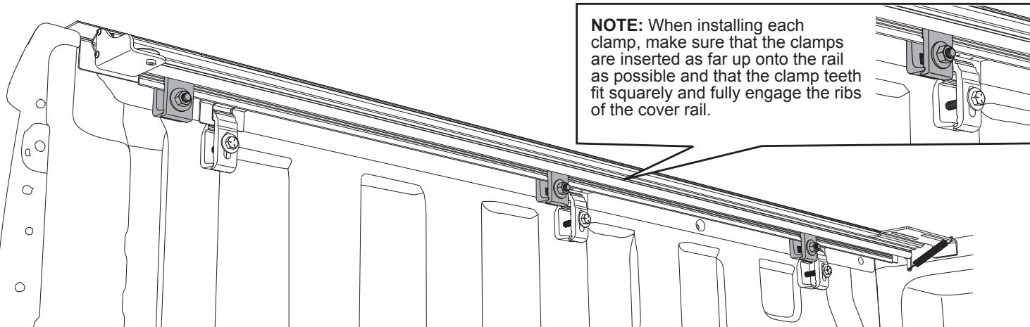
**Repeat steps 1 through 4 for the passenger side add-on rail (E) and the passenger side cover rail (A).**
