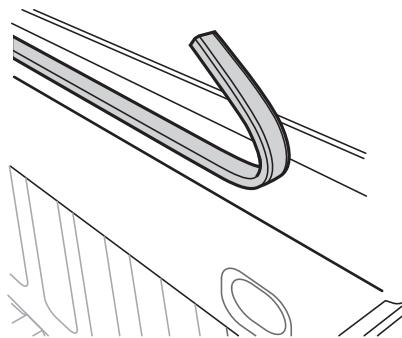
**6** With both rails clamped in place, rest the rolled cover (C) onto the rails at the tailgate, roll the cover toward the cab, and remove and discard all packaging materials.
