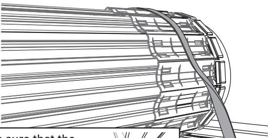
Always make sure that the clamps are inserted as far up onto the cover rail as possible and that the clamp teeth fit squarely and fully engage the ribs of the cover rail.
