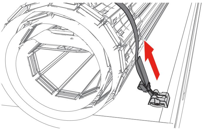
**CLOSING COVER:** Roll the cover (C) toward the tailgate and rotate the tail rail downwards towards the rotating locking levers.
