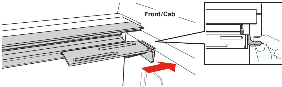
**NOTE: Some drop-in bedliners may require trimming in the corners to fit the rail into the opening**
