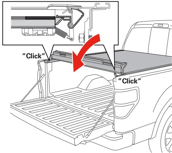
**OPENING COVER:** Pull down on the latch release cable located on either side of the cover (C) and rotate the tail rail forward and into a rolling motion. When driving with the cover open, the cover must be rolled toward the cab and secured with **BOTH** strap clamps.
