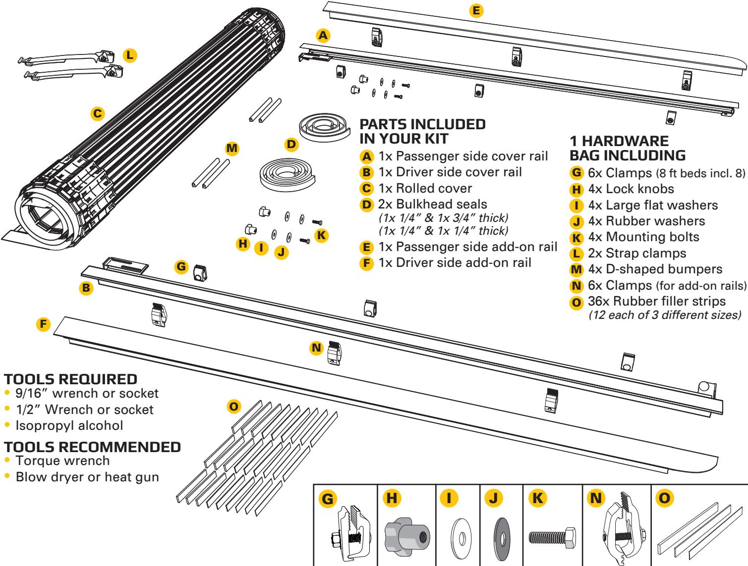
**1** Take the driver side add-on rail (F) and position it into place—the curved portion goes to the rear of the bed.
