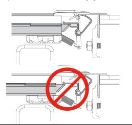
When the cover (C) is properly aligned, roll it open, ensuring not to misalign while opening, and tighten the knobs (H) on both sides to secure the cover. **DO NOT overtighten**. Hand tighten only. Recheck that the cover operates correctly. Close the cover and check that the locking levers are engaged and prevent the cover from being lifted on both sides.
