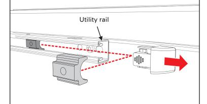
Install a strap clamp (L) to the passenger side adaptor rail (E) near the front/cab with a T-nut kit (N) (a bolt, lock washer, washer, and t-nut). Position the passenger side adaptor rail (E) about a half an inch from the front/cab. Adjust the t-nut so it is lined up with the hole in the adaptor rail. Do not use the big slotted hole and leave loose at this time.
