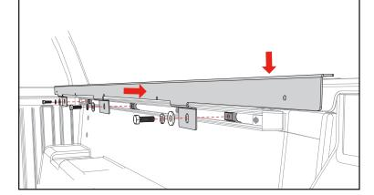
After you get the adaptor rail and the T-nut kits lined up, you can now tighten the bolts, while you are applying downward pressure to the rail (E). Tighten to 10 ft/lbs of torque with a 1/2" wrench or socket. A second set of hands may help. Repeat on the opposite side with the passenger side adaptor rail (F).
