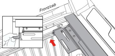
**NOTE**: Some drop-in bedliners may require trimming in the corners to fit the rail into the opening.
