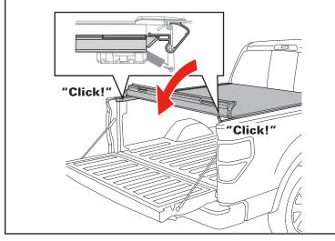
**OPENING COVER:** Pull down on the latch release cable located on either side of the cover (C) and rotate the tail rail forward and into a rolling motion. When driving with the cover open, the cover must be rolled toward the cab and secured with BOTH strap clamps.
