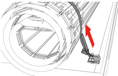
**CLOSING COVER:** Roll the cover (C) toward the tailgate and rotate the tail rail downwards toward the rotating locking levers.
