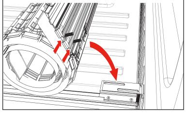
Install the mounting hardware loosely underneath the slotted bracket on the passenger cover rail (A). Start with the rubber washers (J), then the large flat washers (I), then hand tighten the knobs (H). Repeat on the driver side. Leave the knobs loose for now.
