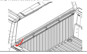
Position the passenger side cover rail (A) on the adaptor rail with the slotted bracket pushed all the way toward the front/cab and touching the cargo rail. If the truck is equipped with a drop-in bedliner, remove the foam pads located at the front of the slotted brackets.
