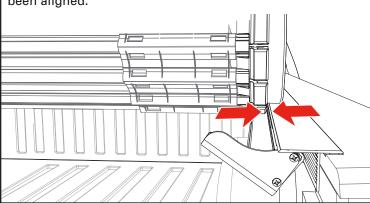
When correctly installed, the vinyl edges of the cover (C) will align squarely with the cover rails in all four corners. The latch assembly will align with the rail locking levers at the tailgate on both sides.
