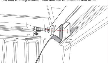
Install the rest of the adaptor rail (E) with the T-nut kits (N). Adjust the t-nuts so they are lined up with the holes in the adaptor rail. Do not use the big slotted holes and leave loose at this time. Repeat steps 2-3 on the driver side with the driver side adaptor rail (F).
