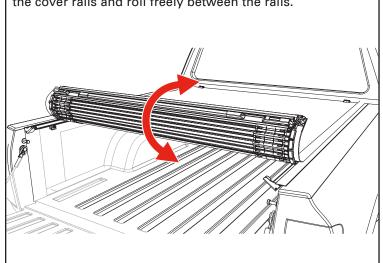
Align the front vinyl edge of the cover (C) with the front edge of the cover rails (not the rubber seal).
